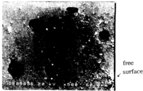
Fig. 3 SEM micrograph showing typical spheroidal cavities in S55C ( \times 500 )
